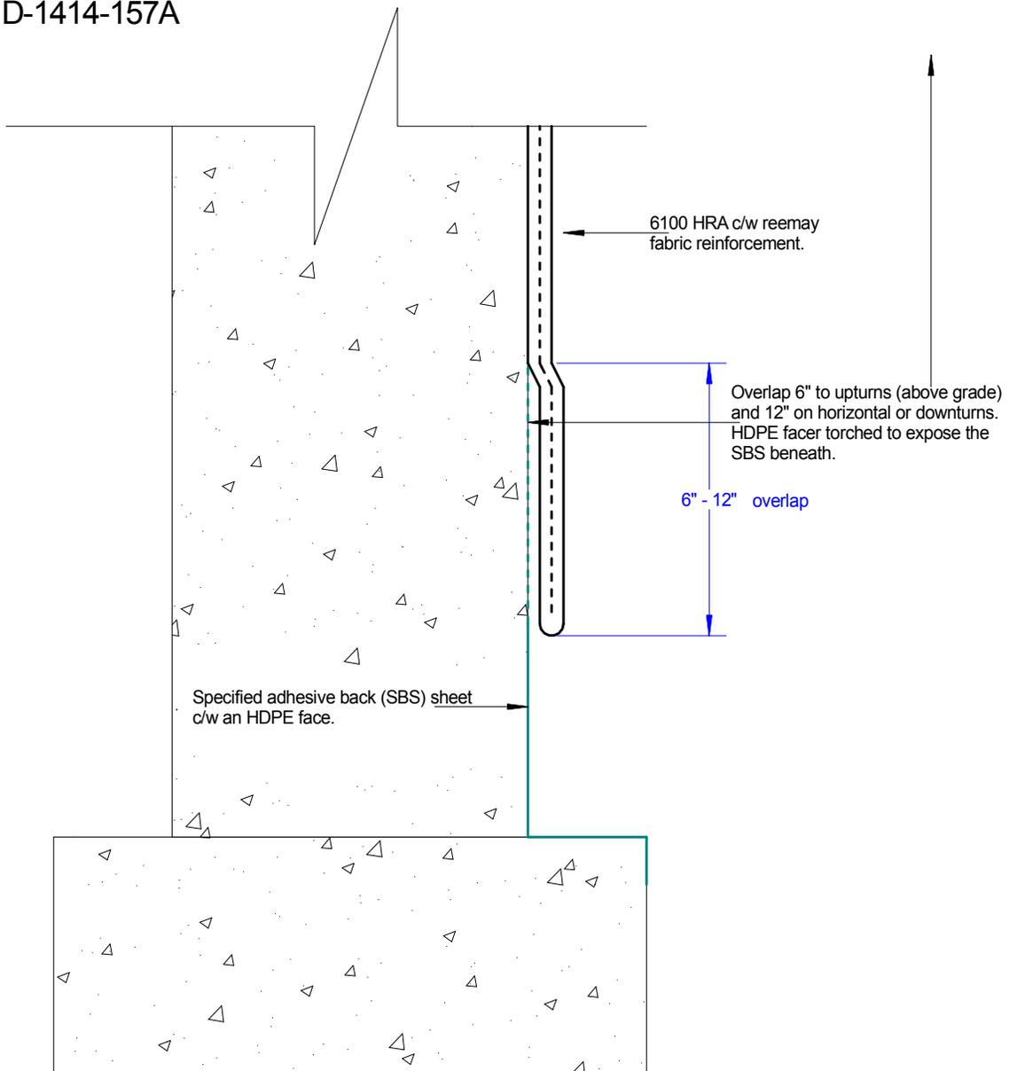
**Note:** To adhere 6100 to the HDPE surface, torch the HDPE to 50% - 75% damage. The 6100 HRA hot rubberized membrane will do the rest. Adhesive back sheet is normally SBS rubber membrane as is the TP-6100 HRA from Tremco. The bond will be more than substantial. No need to prime the adhesive back sheet.
