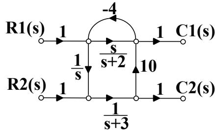
$$T_{11} = \frac{C_1(s)}{R_1(s)}$$
