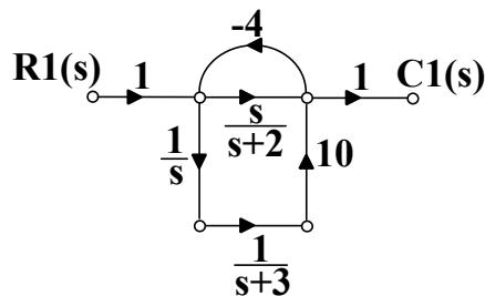
$$T_{11}(s) = \frac{\left(\frac{s}{s+2}\right)(1) + \left(\frac{10}{s(s+3)}\right)(1)}{1 - \left(\frac{-4s}{s+2}\right) - \left(\frac{-40}{s(s+3)}\right)}$$
