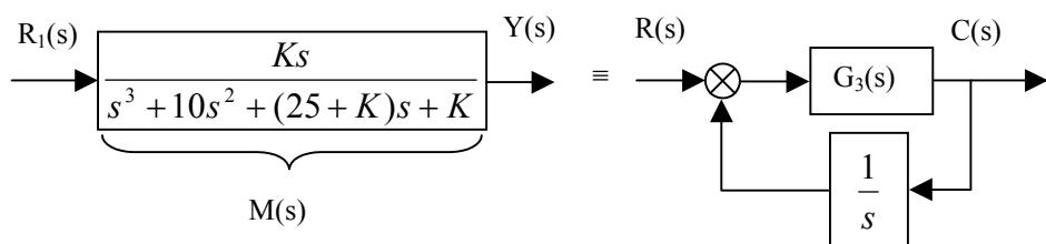
$$M(s) = \frac{G_3(s)}{1 + G_3(s) \cdot \frac{1}{s}} = \frac{s \cdot G_3(s)}{s + G_3(s)} \Rightarrow G_3(s) = \frac{s \cdot M(s)}{s - M(s)} = \frac{K}{s^2 + 10s + (25 + K)}$$
