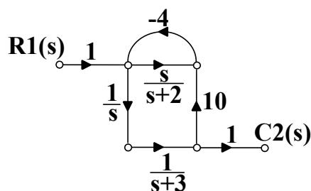
$$T_{21}(s) = \frac{\left(\frac{1}{s(s+3)}\right)(1)}{1 - \left(\frac{-4s}{s+2}\right) - \left(\frac{-40}{s(s+3)}\right)}$$
