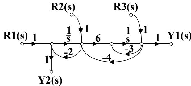
$$T_{11} = \frac{Y_1(s)}{R_1(s)} \quad T_{12} = \frac{Y_1(s)}{R_2(s)}$$
